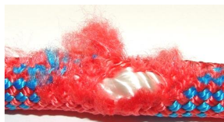
Excessive Abrasion / Wear Contrasting Core visible
