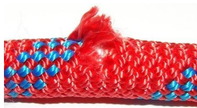
Broken or Cut Strands
