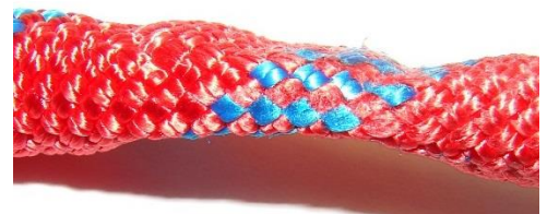
Inconsistent Diameter / Compacted Area
